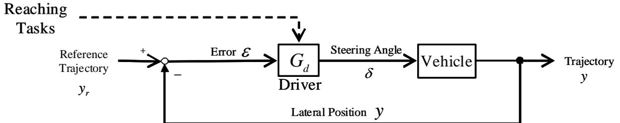
Fig. 3 Driver-Vehicle Model with Reaching Tasks
