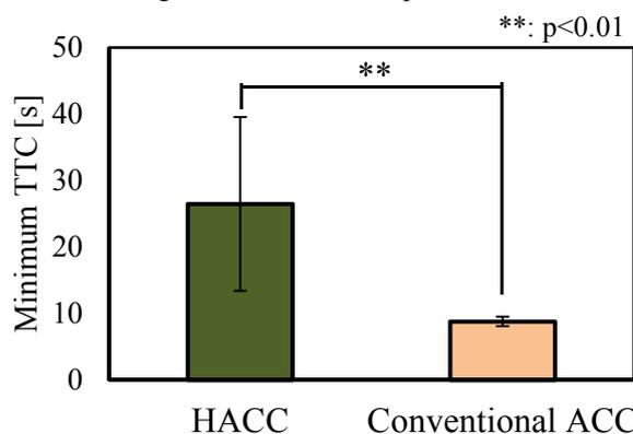
Fig. 6 Minimum TTC from False detection
