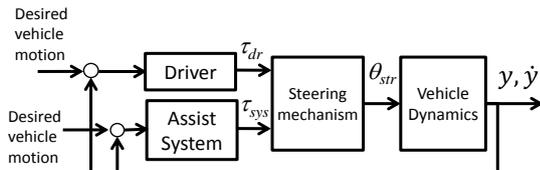
Fig. 1 Block diagram of driver-steering system
