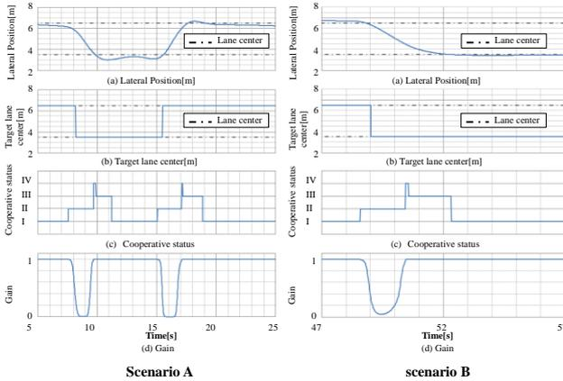
Fig. 2 Plots of the gain-tuning control system responses
