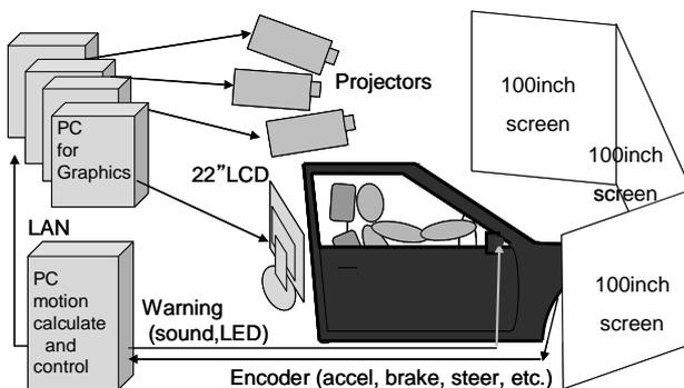
Fig. 6 Composition of driving simulator
