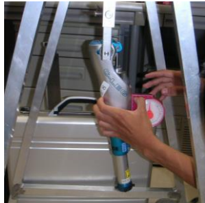
Fig. 5 Measurement of Moment of Inertia.
