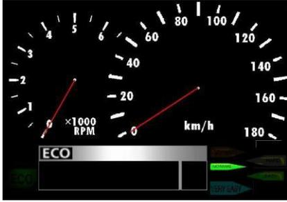
Fig. 3. Instrument Panel Interface Design of the Driving Simulator with Adaptive Assist System. The right hand side of the eco-driving indicator denotes the current level setting.
