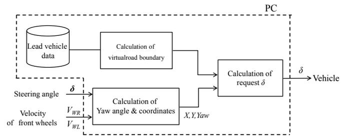
Fig. 8 Experimental system configuration
