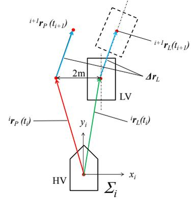
Fig. 2 Relative position of LV and virtual road boundary
